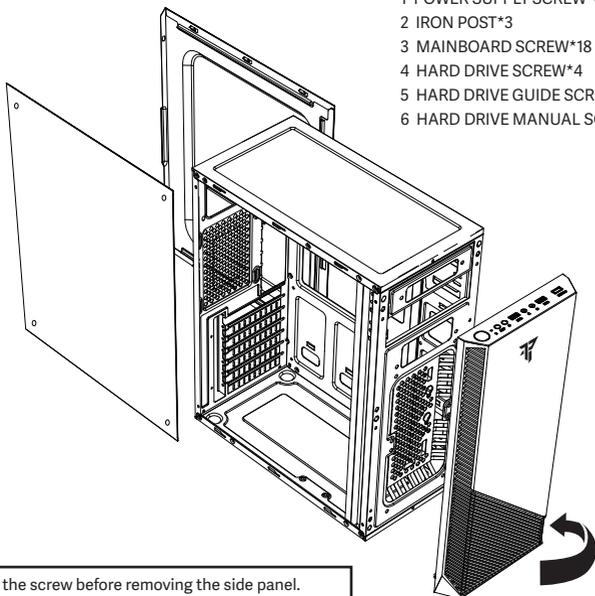
Remove the screw before removing the side panel.
